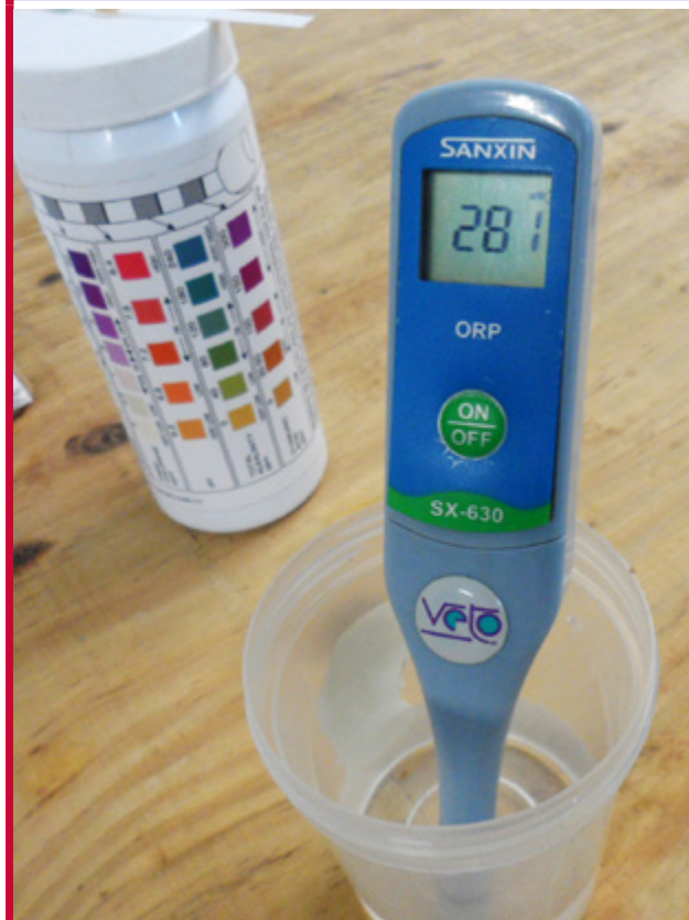
Figure 122 An example of an ORP meter.
