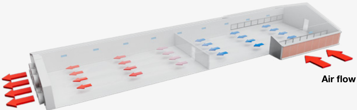
Figure 108 Air flow in a tunnel ventilated house.
