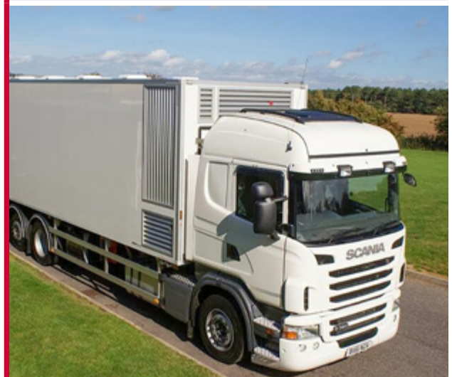
Figure 7 Typical controlled-environment chick delivery vehicles.
